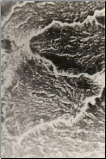
Pic.14. Material Structure of 1,05 Permeability
