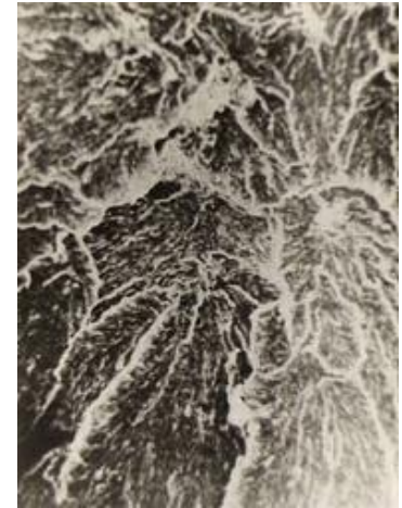
Pic.16. Material Structure of 1,35 Permeability
