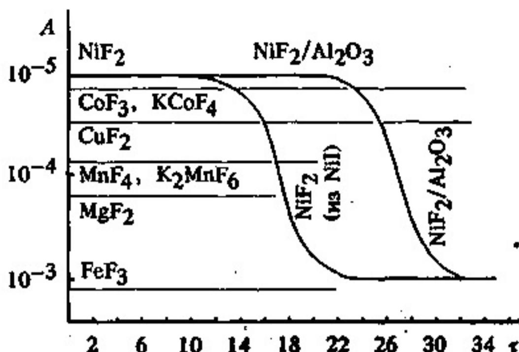
**Fig.2.** Catalytic Fluorination of Hydrogen Containing Admixtures of the Perfluorotributyl material" (Temperature 420 °C, contact period 13 min., A - amount of ion-fluoride bound (process period (h) )
