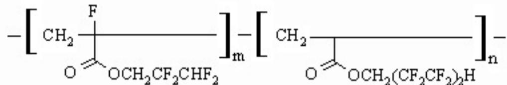
Refraction index of polymer optical fiber is rather low ( $n^{20}_D = 1.4$ ), flow index of melt for applying a light reflecting covering is 10-30 g /10 min at 190 °C. They are well adhesion to the nucleus of this co-polymer, also their elasticity is high. This allows to obtain optical fiber of 2 mm diameter, standing strong flexure.
