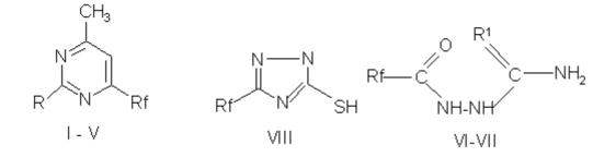
Rf= a C6F13 , b- C8F17 , c - CF(CF3)OC3F7 , d - CF(CF3)[OCF2CF(CF3)]2 , e- CF(CF3) [OCF2(CF3)]nOC3F7 (n=9)
