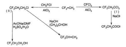
As a result Trifluoropropanes (I, II) being formed are easily converted to trifluoropropanol, trifluoropropene and trifluoropropionic acid.
