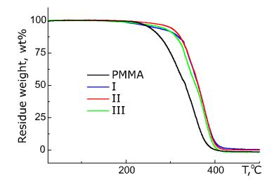
Figure 2. TGA curves of PMMA and PMMA with 2 mol. % of compounds I, II, III.
