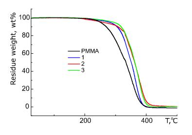
Figure 1. TGA curves of PMMA and PMMA with 1, 2, and 3 mol. % of compound I.
