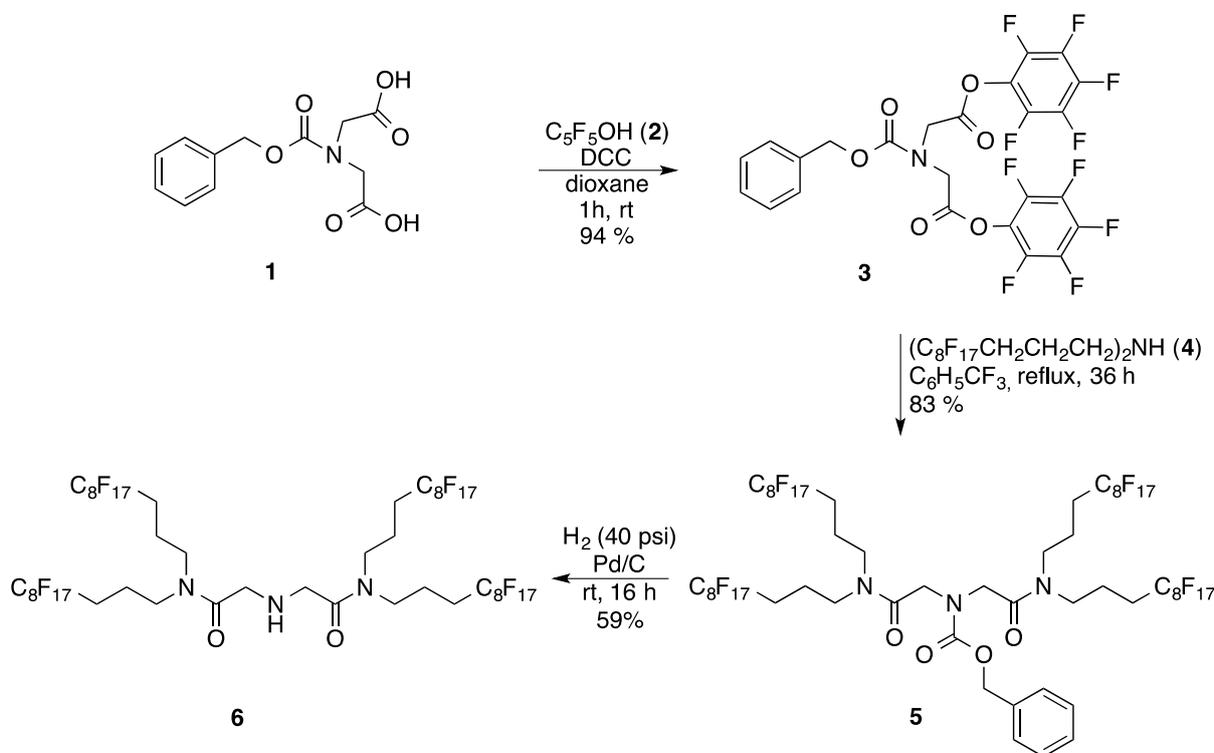
**Scheme 2.** Synthesis of a dendrimer type fluorine 2° amine **6** with four perfluorooctyl-chains.
