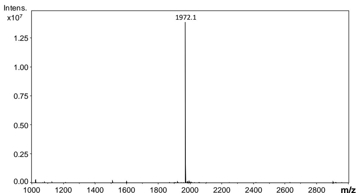
**Figure S1.** ESI-MS spectrum of **6** acquired on a Bruker Daltonics Esquire 3000 plus (Germany) ion trap mass spectrometer. The sample was dissolved in acetonitrile-trifluoroethanol solvent mixture (50:50, V/V). The detected ion corresponds to the protonated molecule  $[\text{M}+\text{H}]^+$ .
