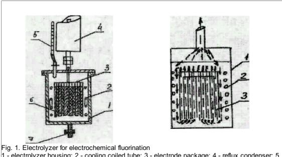
1 - electrolyzer housing; 2 - cooling coiled tube; 3 - electrode package; 4 - reflux condenser; 5 - feed line for organic substrate; 6 - fluoroplast-4 gaskets; 7 - discharge valve.
