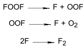
The energy of breaking the FO-OF bond is 103 kcal/mol and only 18 kcal/mol for the F-OOF bond.
